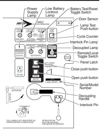
indicate the current switch position. The illuminated buttons indicate the switch position remotely and locally, whether operated manually or by the motor.
