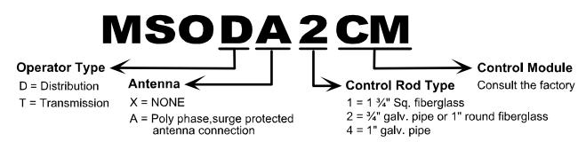
**MSODA2CM** is a motorized switch operator for distribution switches (15 kV-35 kV) with a surge suppressed antenna connection that can be used with either <sup>3</sup>/<sub>4</sub>" galvanized pipe or 1" round fiberglass
