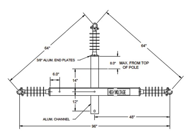
3/4"X 1-3/4" GRADE 5 HEX BOLTS AND LOCK WASHERS SUPPLIED WITH 34.5 KV TINNED UNIVERSAL CLAMP TYPE SILICONE INSULATORS.
