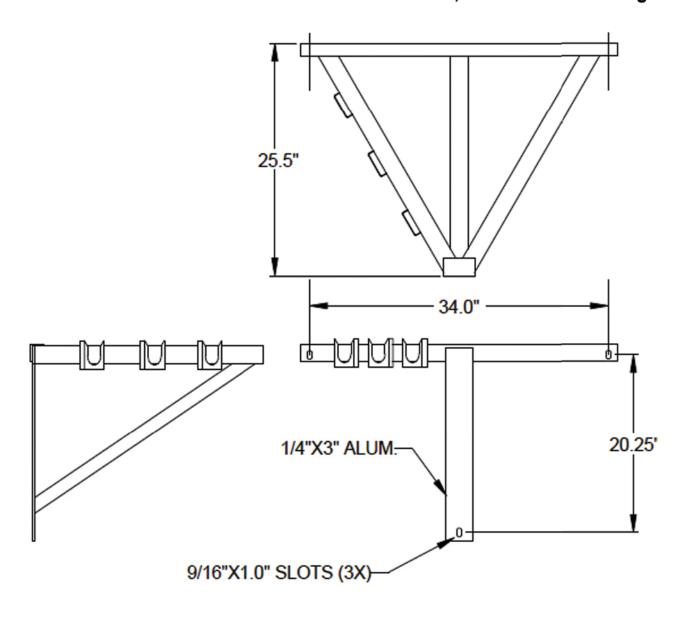
MATERIAL: 6061 ALUMINUM FRAME 304 STAINLESS LOADBREAK ELBOW PARKING STANDS STAINLESS STEEL FASTENERS
