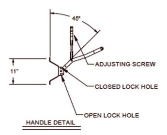
NOTE: RECIPROCATING CONTROL MECHANISM SHOWN. TORSIONAL "SWING HANDLE CONTROLS ARE AVAILABLE.
